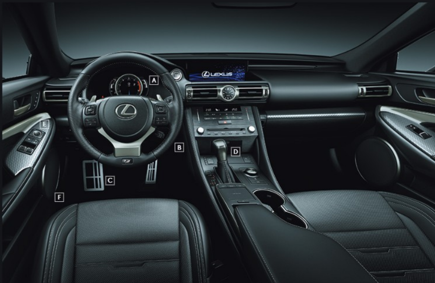
A_Single central meter / B_Steering wheel / C_Aluminum pedals / D_Shift lever knob / E_Trim / F_Scuff plates
